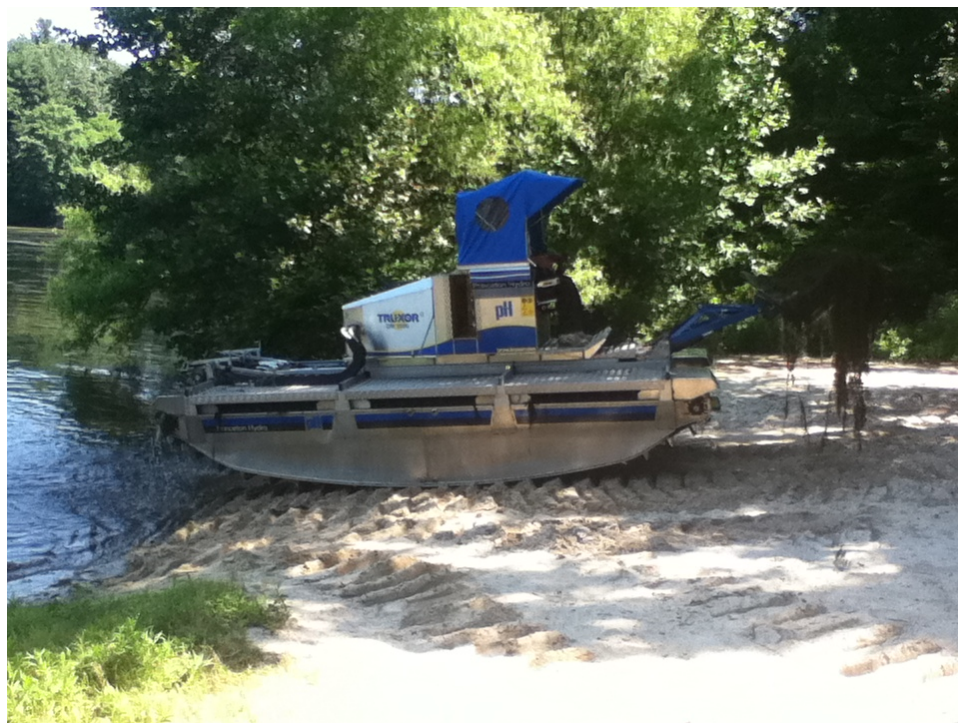
Figure 1: The Truxor, an amphibious aquatic harvesting machine
